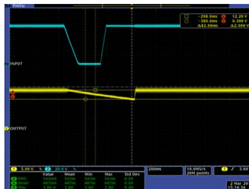
FIGURE 41. CH1: OUTPUT VOLTAGE, CH2: INPUT VOLTAGE
