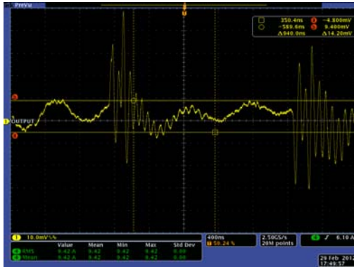
FIGURE 10. 36V INPUT, FULL LOAD, 14.2mV, CH1, OUTPUT VOLTAGE
