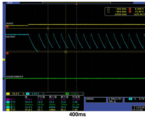
FIGURE 44. CH1: INPUT VOLTAGE, CH2: OUTPUT VOLTAGE, CH4: LOAD CURRENT
