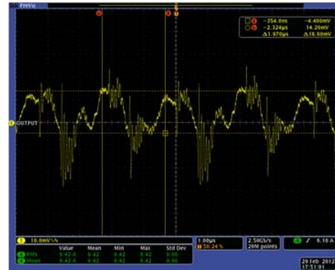
FIGURE 11. 48V INPUT, FULL LOAD, 18.6mV, CH1, OUTPUT VOLTAGE
